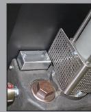
Our patented MOD technology applies heat from the bottom of the hopper up to melt only the adhesive needed, reducing energy consumption and exposure to air, a major source of char. Char is the leading cause of clogged filters/nozzles and premature hose failures that result in downtime. An additional independently heated manifold reduces warm-up time and ensures accurate adhesive delivery temperature.
