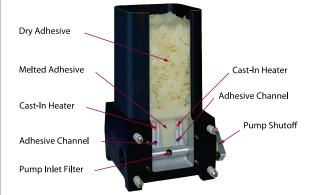
Patented Melt-On-Demand Technology heats from the bottom up, melting only the adhesive needed to prevent charring and degradation. The added benefits of melting only the adhesive required are quicker start-ups, reduced energy costs, better viscosity control, and reduced fumes.
