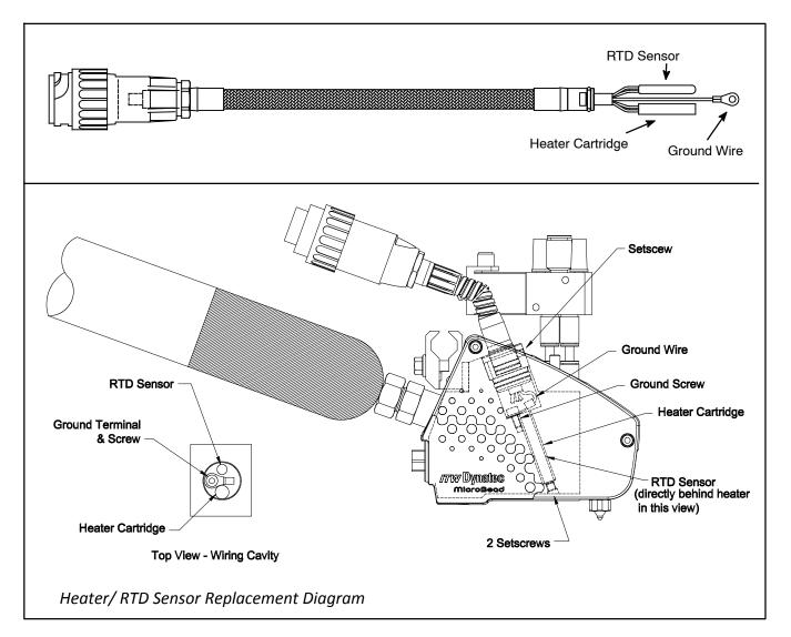
1. Disconnect power to the ASU and make sure all adhesive air pressure and pumps are turned OFF.
